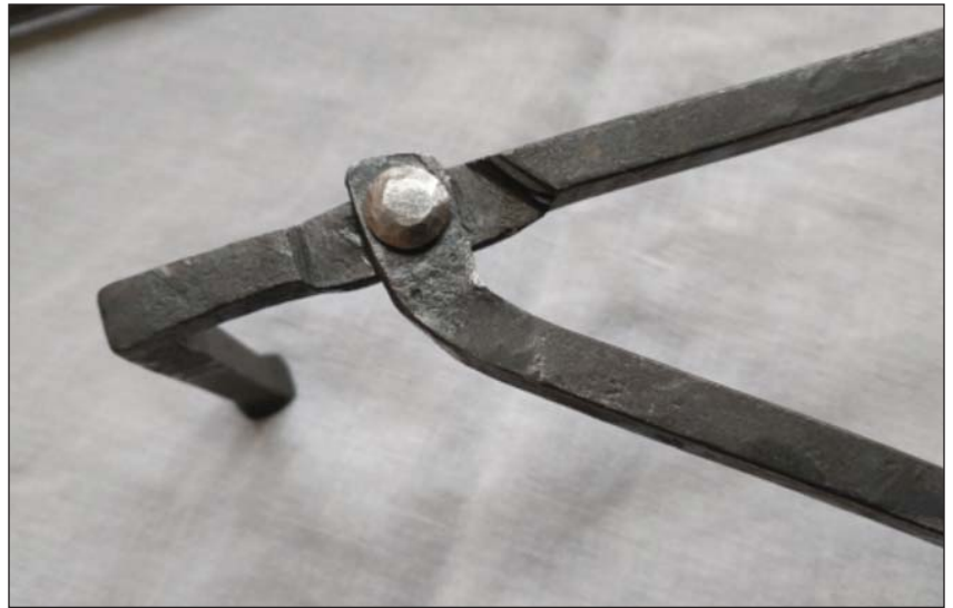
Left to Right - Completed trivet with 90 degree legs and upset feet. Fullered hinge with rivet. Notice the “upset” foot of the trivet with the wider base.
