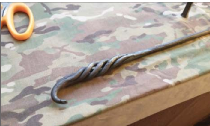
Left to right – Basket handle of the fire poker and the “Working” end of the fire poker. Both the handle and the working end of the fire poker were completed using the “forge welding” technique.
