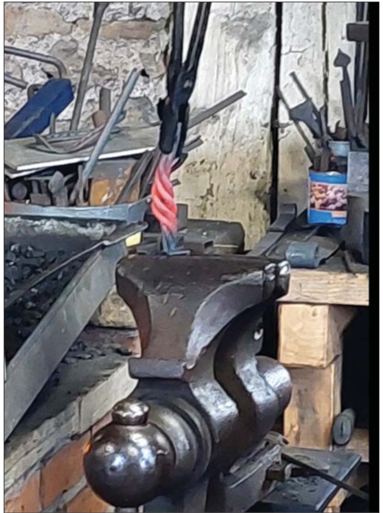
Left to right - Spiral handle and working end of the fire poker. A basket handle receiving the twist with the help of a vice and a pair of tongs.
