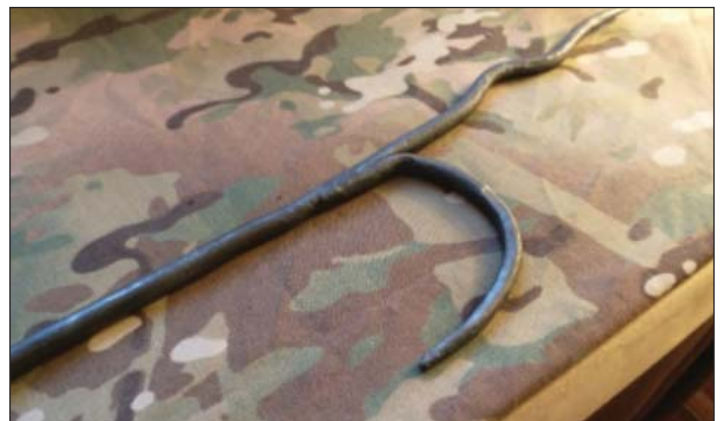
Left to right – Basket handle of the fire poker and the “Working” end of the fire poker. Both the handle and the working end of the fire poker were completed using the “forge welding” technique.
