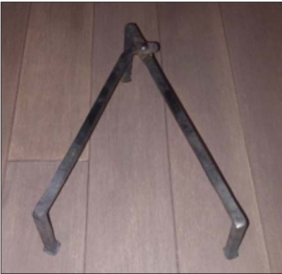
Left to Right - Completed trivet with 90 degree legs and upset feet. Fullered hinge with rivet. Notice the “upset” foot of the trivet with the wider base.
